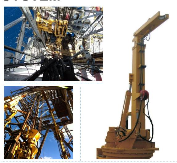
THE GRIPPING AND LIFTING CAPABILITY OF THE BRIDGE RACKING CRANE COMBINED WITH THE CAPTURED GUIDANCE OF THE LOWER RACKING ARM ENABLES VERTICAL STANDS OF PIPE TO BE HANDLED AND GUIDED SAFELY BETWEEN SETBACK TO MOUSEHOLE TO WELL CENTRE
