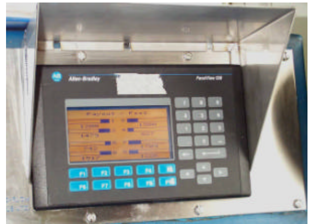
TYPICAL ANCHOR WINCH MONITORING DIGITAL DISPLAYS
